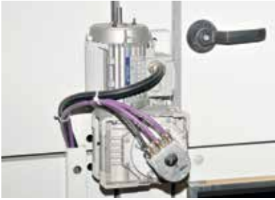
En ayar tahrik sistemi ve mutlak enkoderi / Width control with absolute encode
