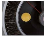
**4 S/Z switch** Used to set the direction of rotation. **5 Yarn speed switch** Used to adjust the yarn speed.
